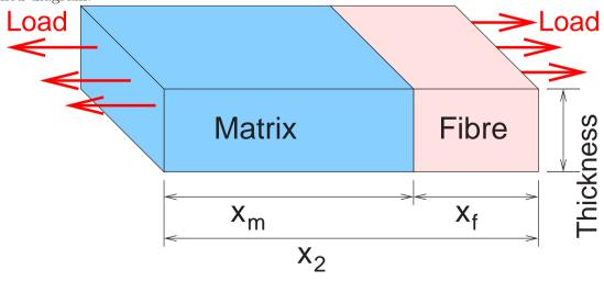
Clearly, the total original length  $x_2$  is just the sum of the original lengths of the fibres and the matrix.
