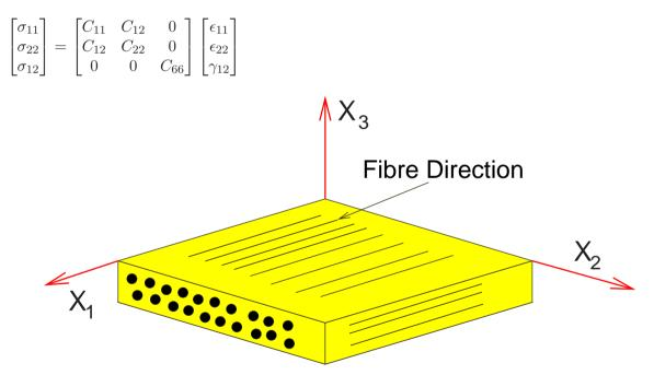
Note that the decoupling of shear/extensional stress/strain is crucial to this step. The plane of the plate has to be closely related to the principle directions of the laminate. Note, corrected from last week.
