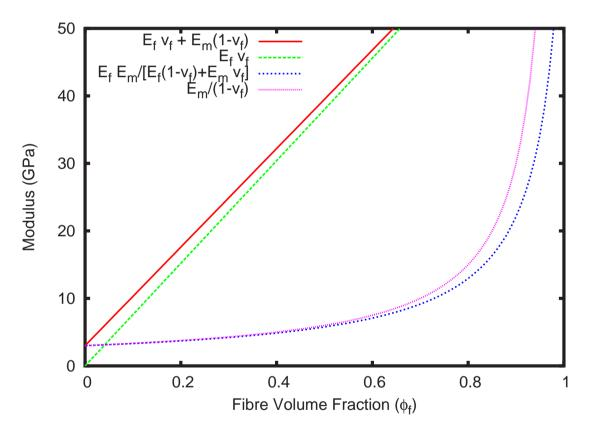
Note that the properties used here for the fibre and matrix stiffness are the same as used in the worked example later in this document, and relate to glass fibre embedded in a polyester matrix.
