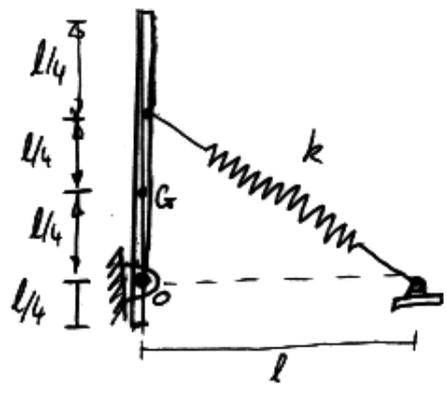
if bar is rotated  $30^\circ$  clockwise, & released, find initial value for  $\alpha$
