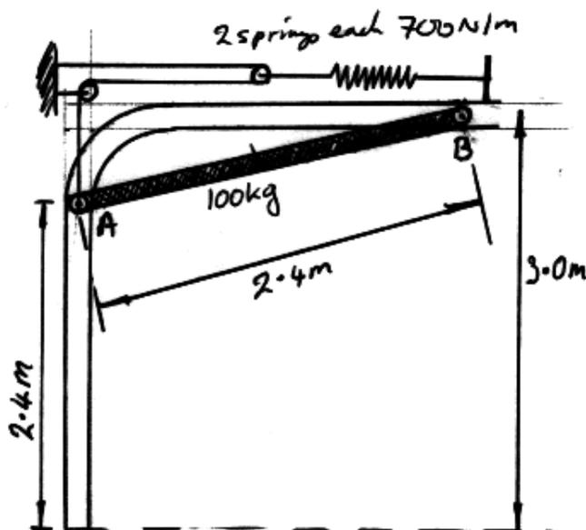
note, as door hits floor, it has no angular velocity since at that moment it is constrained to move straight down.
