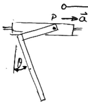
"L" is attached @ P to a slider & the assembly has a constant accln of  $\vec{a}$  as shown. We are asked for steady state values of  $\theta$
