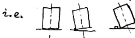
note, the force  $\vec{R}$  is, in GENERAL, distributed over the bottom of the cylinder, but once it starts to tip, the bottom surface lifts clear and all of  $R$  occurs at A
