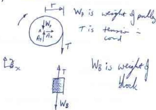
for pulley  $\Sigma M_A = I_A \alpha$
