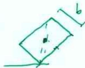
$$\frac{1}{2} I_0 \omega^2 - mg \left[ \sqrt{\left(\frac{b}{2}\right)^2 + \left(\frac{c}{2}\right)^2} - \frac{b}{2} \right] = 0$$
