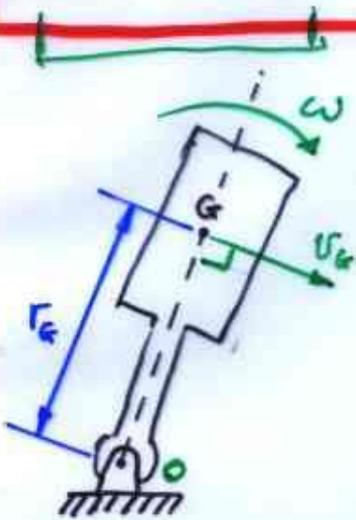
note  $\vec{v}_G$  must be perpendicular to  $\vec{r}_G$  due to kinematics
